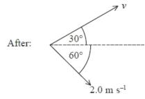
(i) Show that the magnitude of the velocity v of the first puck after the collision is about 3.5 m s<sup>-1</sup>.
